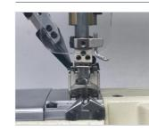
牛角式布诱导器使埋压拷克骨更为稳定。 "Horn type"regulating fabric guide, to offer stable covering stitch.
