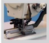
可选用120mm大压脚进行门襟钮扣孔连续两次以上 车缝,提高生产效率 120mm big presser foot is optionally selected to button-hole the Shirt-Fronting continuously, increase the efficiency of productivity
