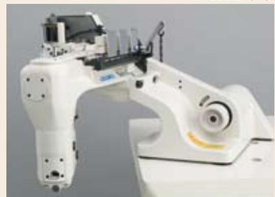
★ To install the machine on the table, the auxiliary drive MT03 is required.
