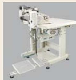
★ This table stand is specifically designed for the SC-510. The M-51 motor should be used.
