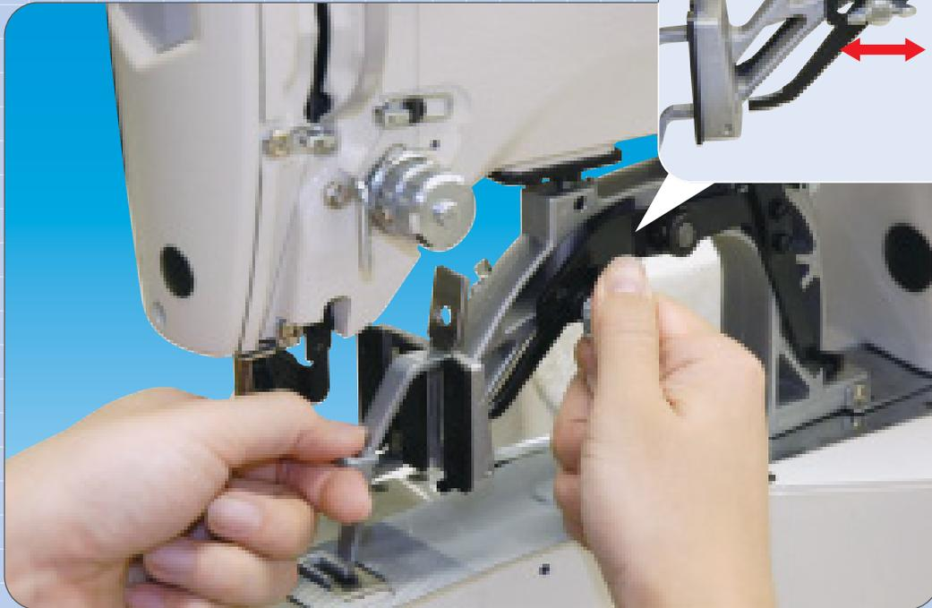
·Conventionally, the front plate has to be removed to change the work clamp. With the new work clamp kit, the work clamp can be changed without removing the plate.
